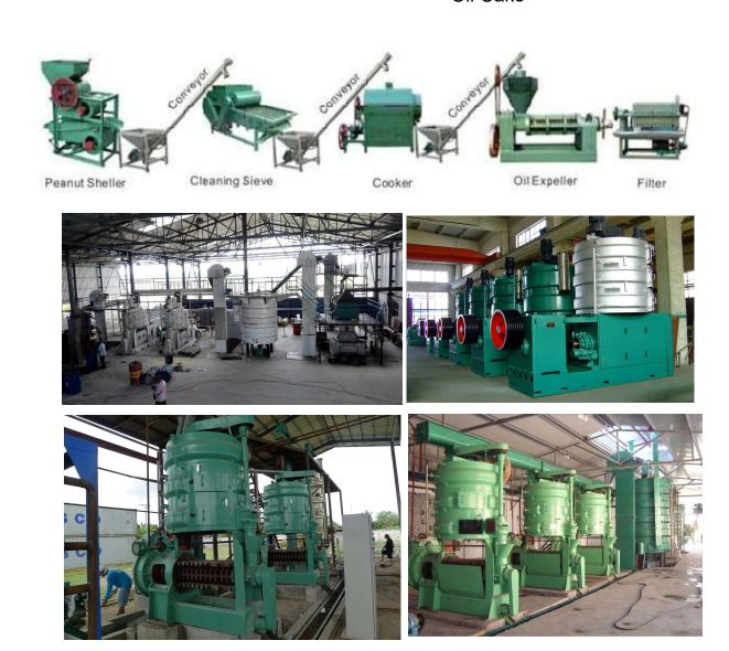
NiveSal can help in setting up low cost oil extraction units from groundnuts or any other locally available oil seeds like Shea nut, Copra etc. Depending on the market requirement we can also provide complete refining system for these oils.
