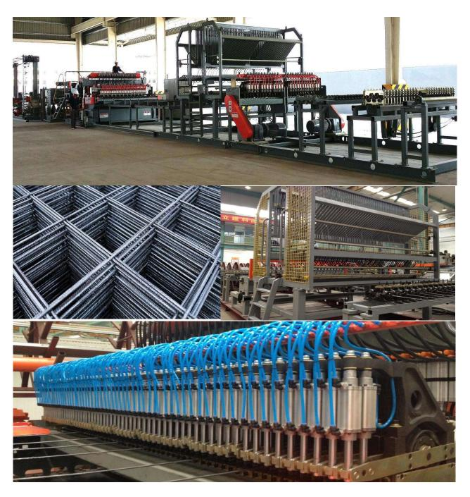
Welded mesh is widely used in construction. With rapid development of roads and prefabricated building technology, this equipment is gaining popularity in all countries because it saves material and site manpower cost. NiveSal provide fully automatic and also semi-automatic options to cater to different market segments in terms of investment and output capacities.
