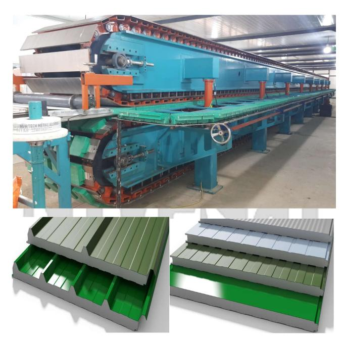
NiveSal takes turnkey contract to design supply and install complete Sandwich Panel Lines for different industries. From regular industrial roof and wall panels to most sophisticated cold box panels. The lines can be customised to exact requirents for each client for PU or PIR insunation material, 2 or 5 component chemical foaming system and 18 to 36m press. NiveSal provides the bets combination of technical superiority within economical budget to achieve higher output to investment ratio.
