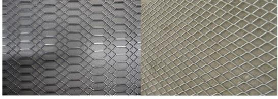
Expanded Metal Mesh is a multi-utility product, used widely in developing countries for wide range of applications from construction to hardware. NlveSal has developed a complete automatic production line capable of producing different designs in the same machine. This line can produce expanded metal mesh from steel coils in coil or sheet from with flattening and levelling options.
