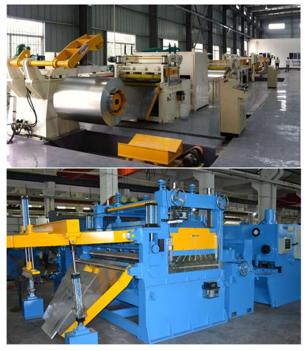
Cut to length line is a primary requirement in any service centre. We provide complete range of cut to length lines for all types of applications. We can provide from lines for thickness range from 0.1mm to 25mm, width up to 2500mm and speed from 20 to 120 meters per minute. We have specialised lines for Steel Mills, Service Centres, Auto Component manufacturers and various other applications.
