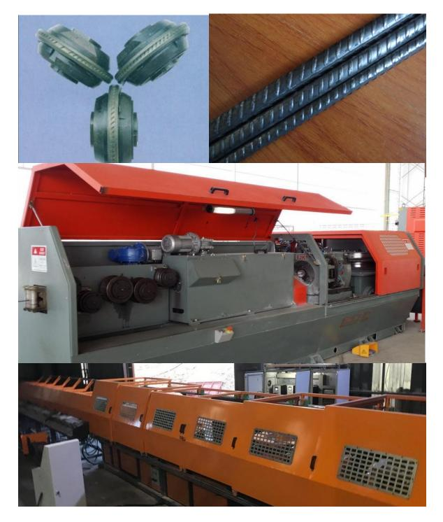
In many developing countries cold forming of rebars is a convenient and cost effective solution. Wire rods of relevant diameters are rolled under rolling cassettes to create the ribs under normal temperature. NiveSal has one of the best solutions for this project providing accurate and fast production of rebars with very reliable and long lasting equipment.
